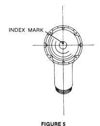
c. Place the cover (26) in position on the second stage housing. Insert the screws (27) and tighten snugly with a screwdriver
